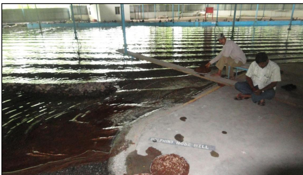
Figure 5.5 Tracer material injection studies for sand trap configuration on Physical Wave Model of Visakhapatnam Port
