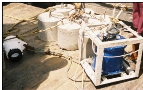
Figure 4.9: Tide Gauge with Acoustic Release
