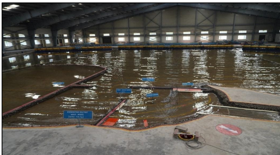
Figure 5.7: Wave tranquillity studies conducted in MPWB for fishing harbour at Vizhinjam Port, Kerala
