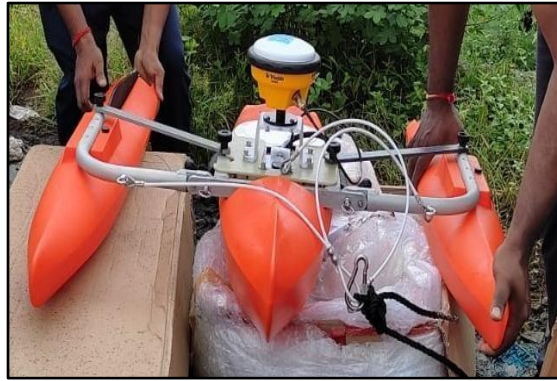
Figure 4.12: River Pro 1200 kHz ADCP along with Trimaran Boat and GNSS antenna
