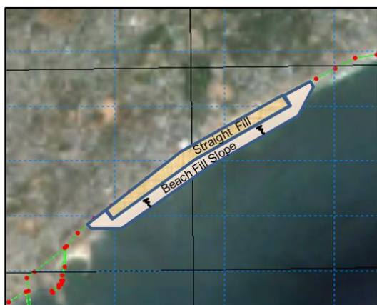
Figure 5.27: Beach fill Design using Coupled model
