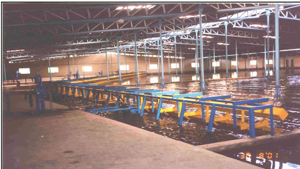
Figure 5.2 Physical Wave Model housed in a MS tubular structure equipped with RSWG system
